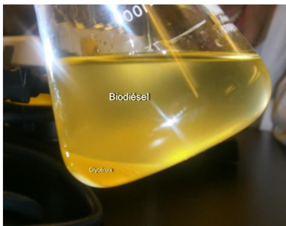
Figure 2: Erlenmeyer flask with two phases (upper: biodiesel, lower: glycerin). Image by Ian Wikarski
